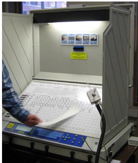
After the second press of the “Cast Vote” button, the VVPAT is ejected out the front.
